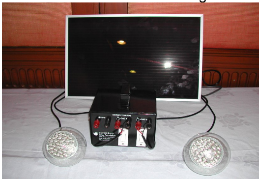
SOLAR LED 33 LEDs - 2 LAMPS & A 10 WATT PANEL
